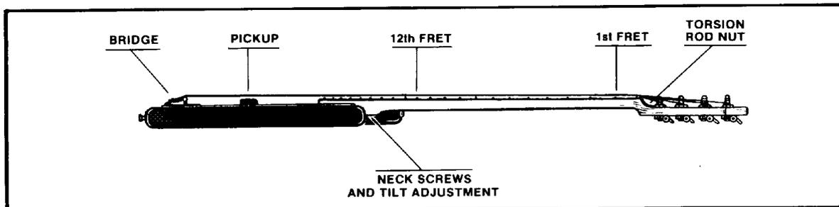
4. String height may now be adjusted with the neck tilt screw, which is located **inside** the small hole in the neck plate. A 1/8" Allen wrench is used to make this adjustment. Turning the screw clockwise raises the end of the neck, thus bringing the strings closer to the fingerboard.
