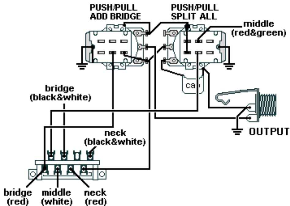
Ground green & bare wires from neck & bridge pickups and black & bare wires from middle pickup.
