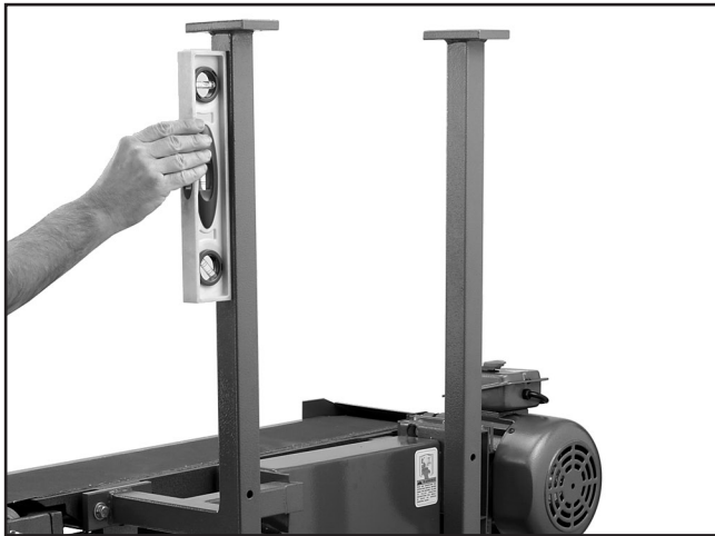
Figure 6. Plumbing the short support bracket.
