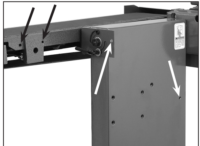
Figure 2. Installation hole locations.
