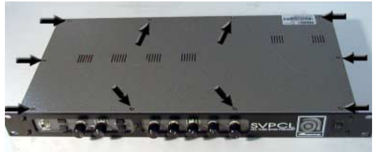
Figure 1: Remove top cover screws
