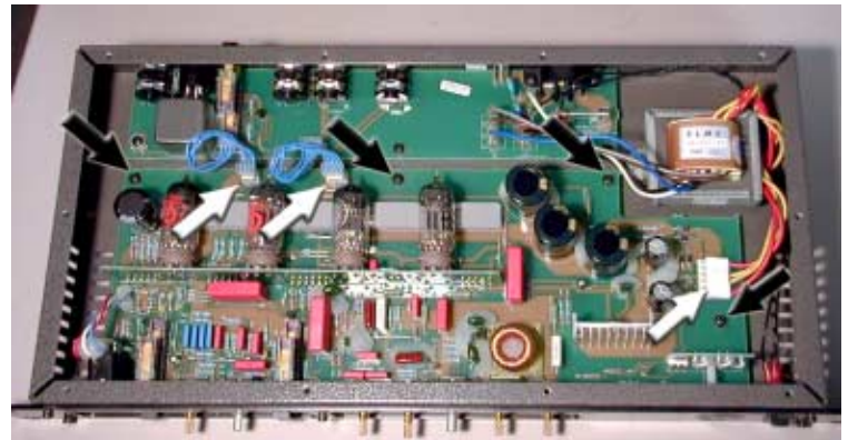
Figure 3: Disconnect harnesses, remove PCB screws
