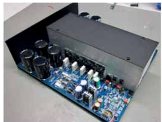
Power amp board with metal board
