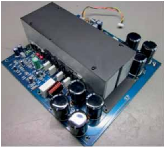
Power amp with metal board removed
