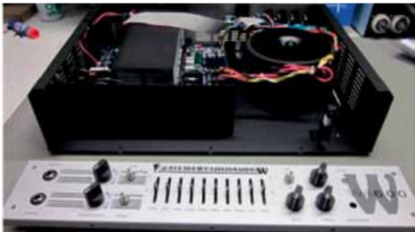
7 screws (3 on the bottom of chassis) are holding pre-amp with front chassis
