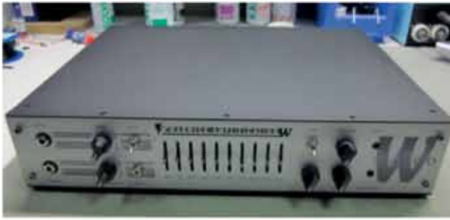
12 screws are holding top chassis of WA600
