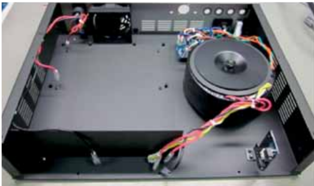
Chassis with transformer, soft start board and metal board for power amp
