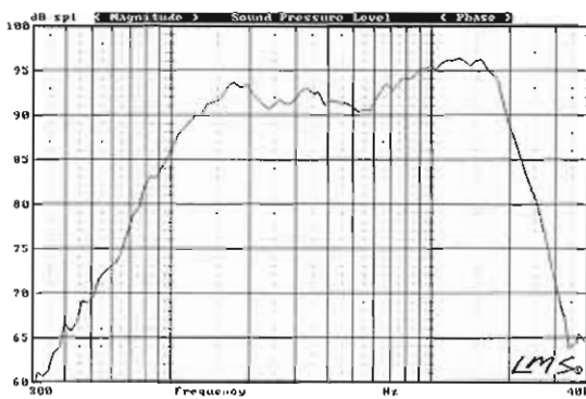
FIGURE 12.57: Surround single tweeter on-axis frequency response.
