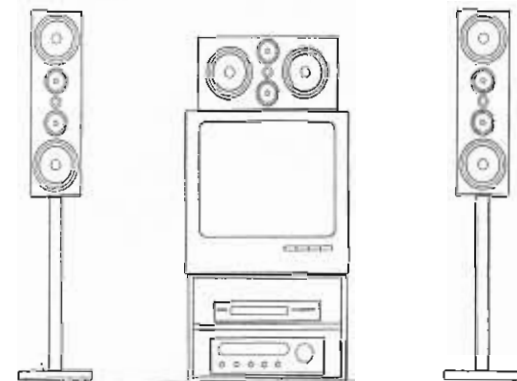
FIGURE 10.21: Controlled directivity three-way speaker format.
