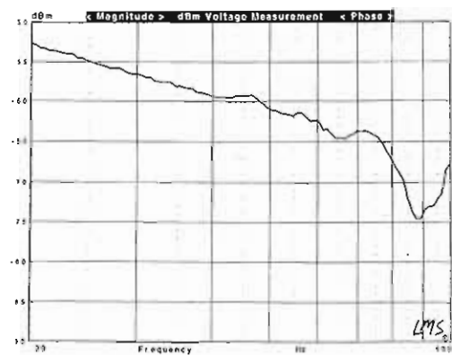
FIGURE 11.4: Measured free-field cone excursion curve.
