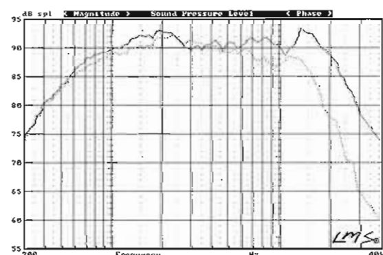
FIGURE 12.90: Studio monitor tweeter on- and off-axis frequency response (solid = 0°; dot = 30°).
