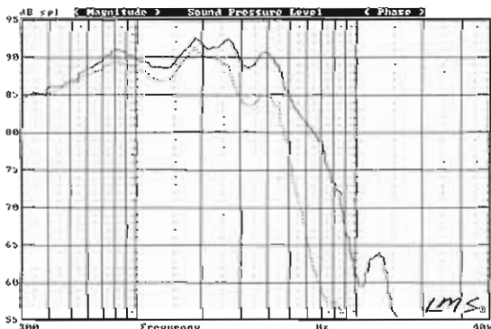
FIGURE 12.87: Studio monitor woofer on- and off-axis frequency response (solid = 0°; dot = 30°).
