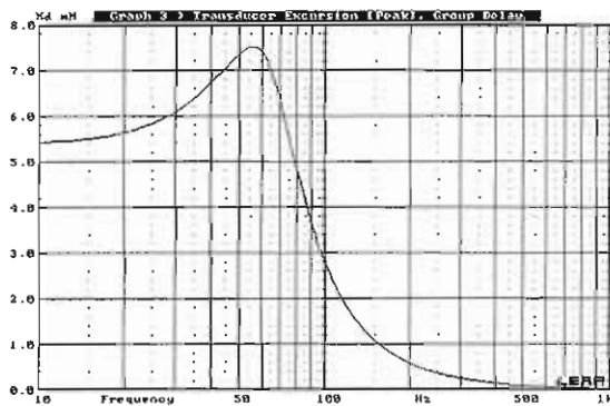
FIGURE 12.83: Cone-excursion curve for the 15.5V curve in Fig. 12.81.
