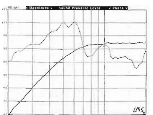
FIGURE 11.7: Comparison of free-field response in Fig. 11.6 with closed-field frequency response.
