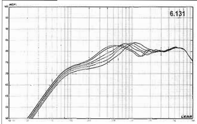
FIGURE 6.134: On-axis frequency response comparison of the largest baffle size with the infinite baffle response (solid = infinite baffle, dash = 40" wide baffle).
