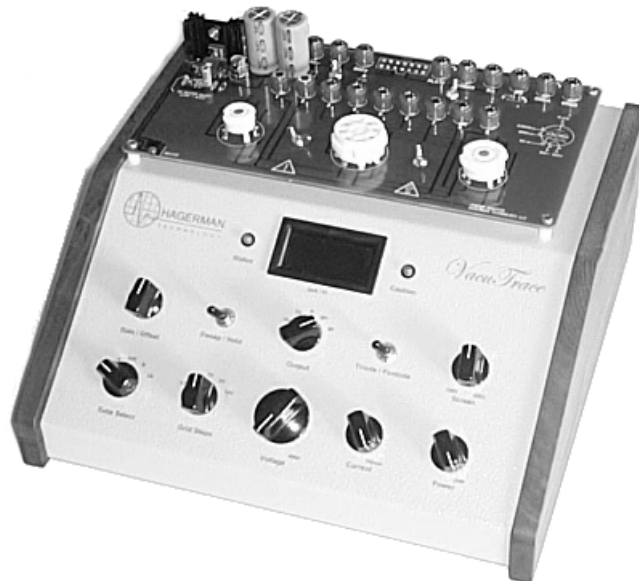
Figure 1. Jumper Adapter Card installed onto VacuTrace.
