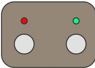
BOTH THE RECORD AND PLAYBACK SWITCHES ARE OFF. THIS IS THE (NON TRUE) BYPASS MODE.
