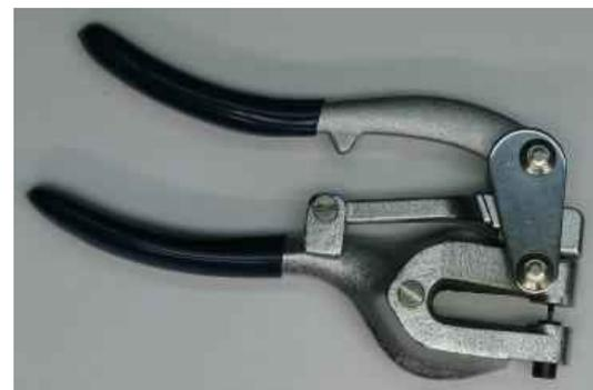
The hand punch is wonderfully easy to store in between uses. The largest downside is the hand punch requires a good bit of physical strength to punch through 1/8" G10 epoxy board. The typical board will have 20+ turrets so that is a lot of work. I admit, after 10 or so turrets, I break into a sweat nearly every time. But for quick construction or when access to a drill is limited, the hand punch tool is a great option.
