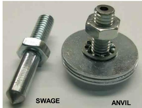
File the threaded end flat and smooth. Then lightly chamfer the edges.
