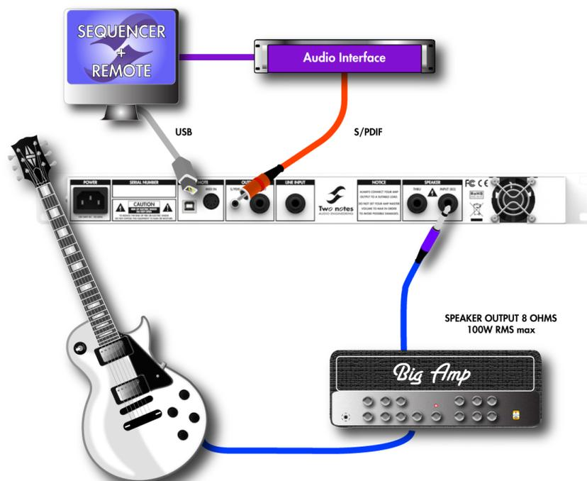
Plug your 8 ohms out on your amplifier to the SPEAKER input of the TORPEDO Live. If you want to use a preamplifier, plug its line output to the LINE INPUT of the machine.
