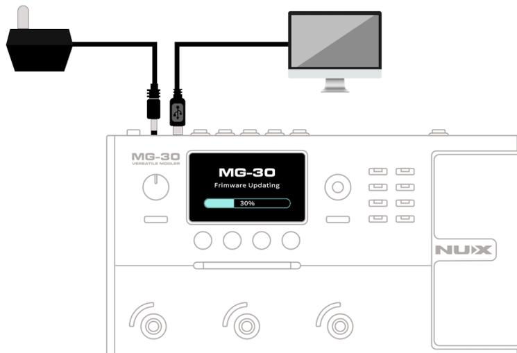
3. When the firmware update process is complete, close "NUX DFU Updater", disconnect the USB-C cable and turn off the power switch.
