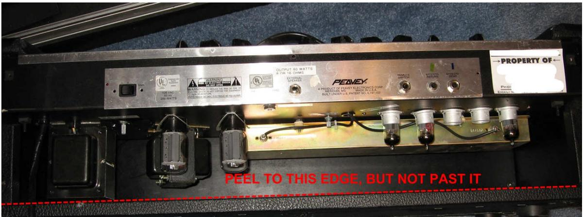
Then put the amp on its side, take a utility knife and cut a seam in the Tolex along the bottom edge of the amp (do this on both sides.)
