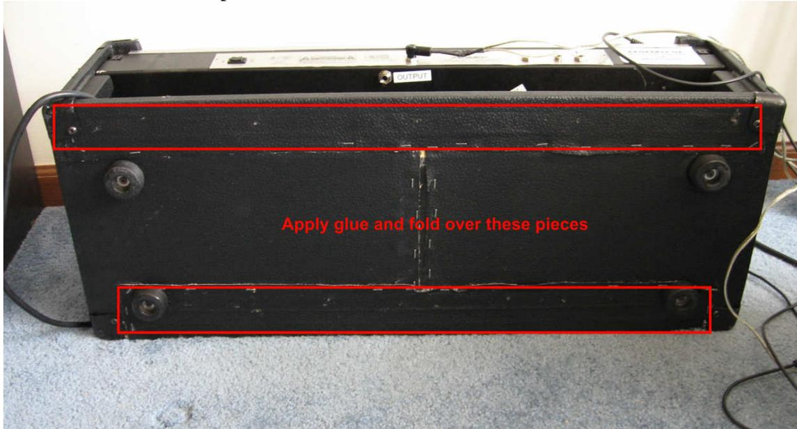
This is the last layer of tolex on the bottom, to really put a bunch of staples around the edges to hold everything in place.
