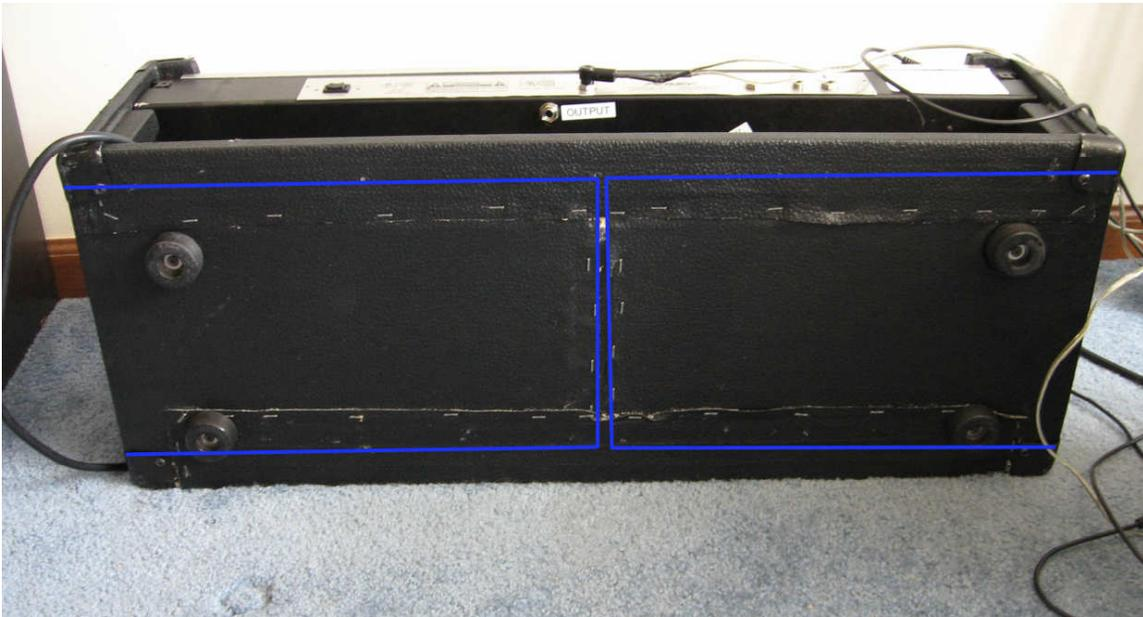
Once the 2 side pieces are glued down, there will be some excess tolex. The blue above illustrates how you should trim the side pieces of tolex with a utility knife IMMEDIATELY AFTER it has been glued down (that way it will come up easily).
