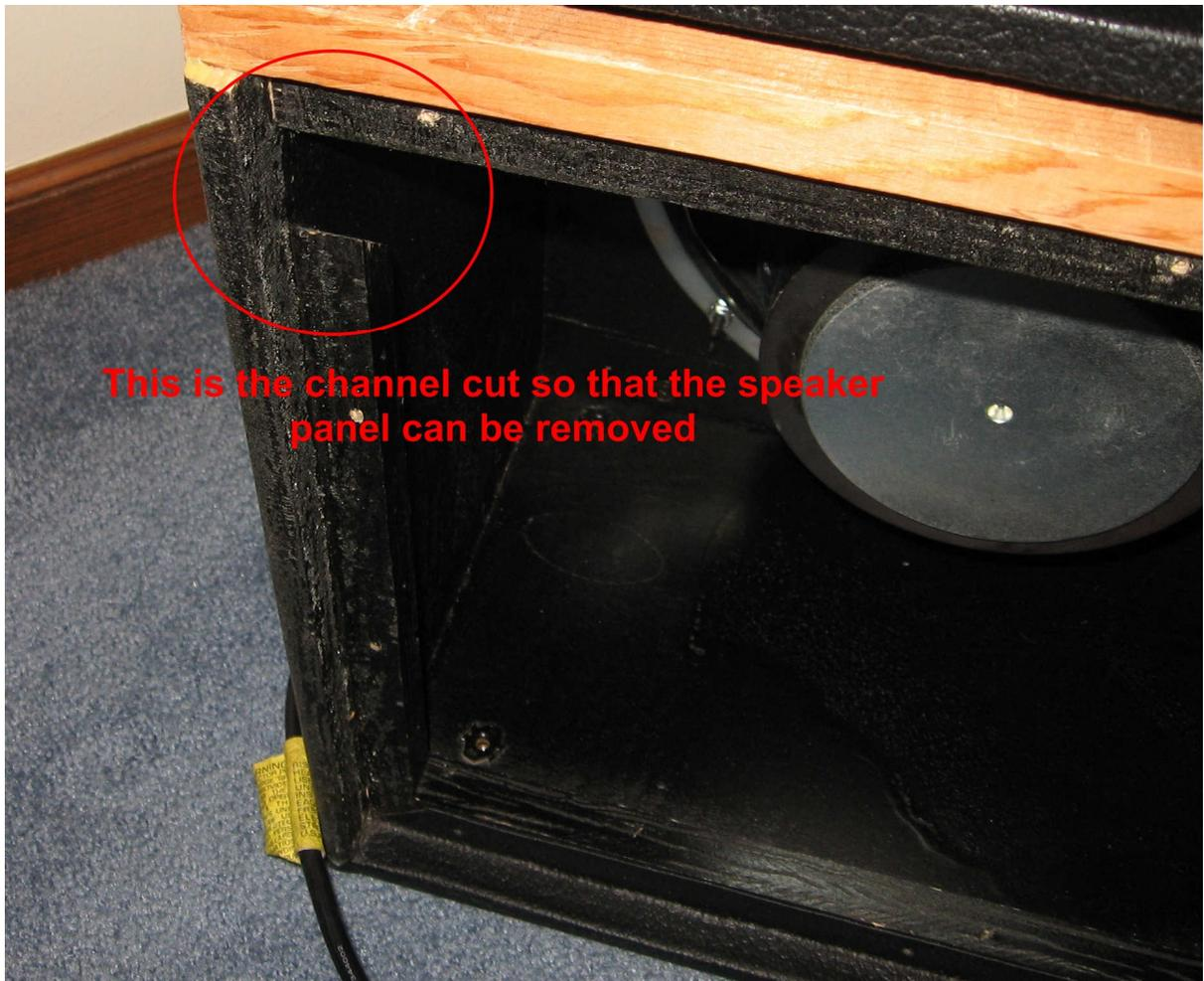
Once the speaker panel is gone, remove the many staples holding the plastic trim piece in around the front of the speaker cab, and remove the trim piece. This is **EXTREMELY** tedious and nasty work, but you have to do it.
