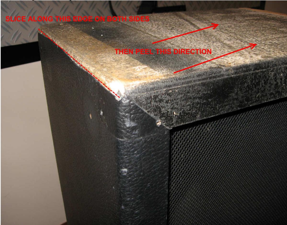
Pull up the Tolex on both sides of the amp and peel it all the up to approximately the level that the tubes hang at
