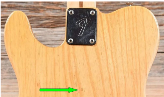
Pin router's hole, 1977 Fender Telecaster. Courtesy of Chicago Music Exchange
