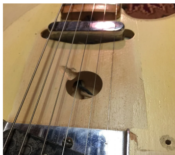
A few "transition" dual pickup guitars, made around February 1951, featured a small "donut" hole in the center of the body, under the
