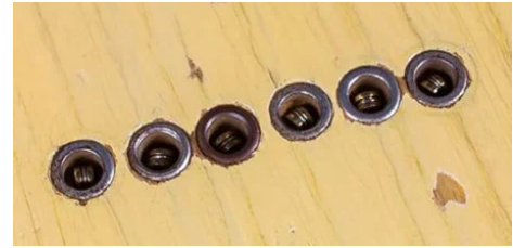
Misaligned holes, 1950 Broadcaster, Courtesy of Garrett Park Guitars
