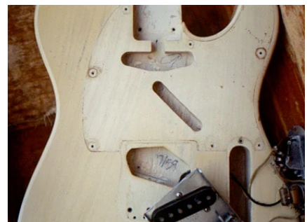
After early 1951, all Telecaster style guitars had cavities for both pickups,
