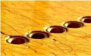
Detail: countersunk holes and flush with the body string ferrules, Courtesy of Eddie Tatton
