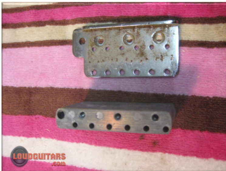
Top plate removed from the tailpiece block.
