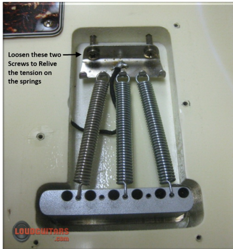
Loosen these two screws to relieve the tension on the springs.
