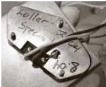
Bill wired the guitar with a 4-way switch using a pair of Jason Lollar's Tele 'Special' pickups and 250K pots for neck, neck/bridge, bridge and combined out-of-phase tones. With a clean amp you can get very close to the tone of a jazz box on the neck pickup, the
