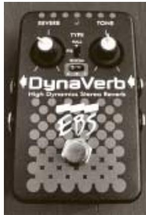
and the third mode is “Hall,” with settings for a “Large Open Hall,” and “Ambience” hall. The DynaVerb can also be operated in stereo mode with two amplifiers or connected to a mixing console in parallel mode and used as a ‘rack’ unit.
