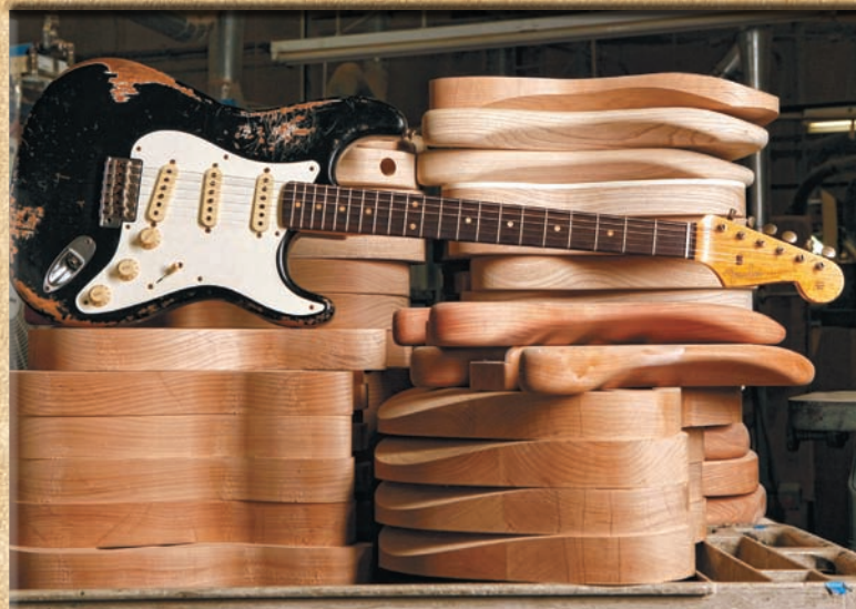
Slab blanks and contoured bodies back up a 2010 Custom Shop 1959 Black Stratocaster. Fender Musical Instruments Corporation
