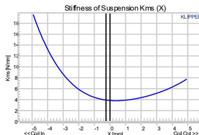
Figure 10: Stiffness  $K_{ms}(x)$  versus displacement  $x$ .
