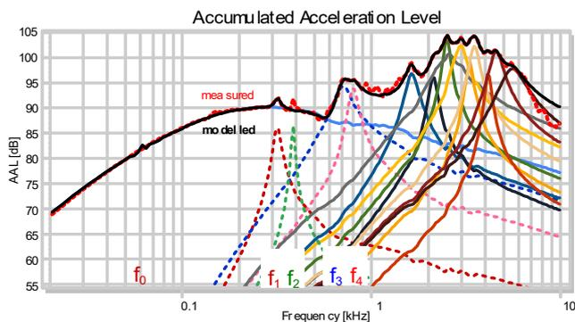
Figure 13: Contribution of the mechanical vibration modes on the radiation surface (cone, surround, dust-cap) to the measured and modelled accumulated acceleration level ( $AAL$ ).
