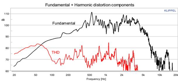
Figure 8: Total harmonic distortion (THD) compared to the fundamental component in SPL generated by a sinusoidal sweep with 25 V<sub>RMS</sub> at the input terminals.
