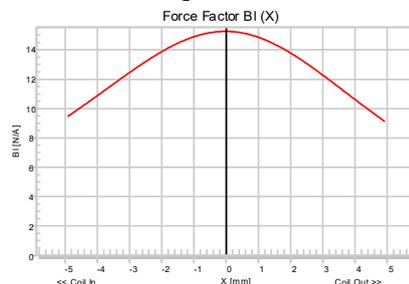
Figure 11: Force factor  $Bl(x)$  versus displacement  $x$ .
