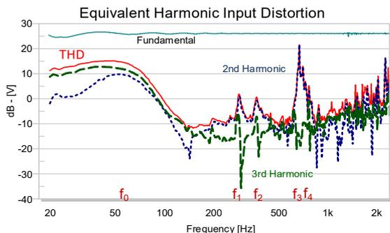
Figure 9: 2<sup>nd</sup>-order, 3<sup>rd</sup>-order components and total harmonic distortion compared to the fundamental component transformed to the loudspeaker input terminals
