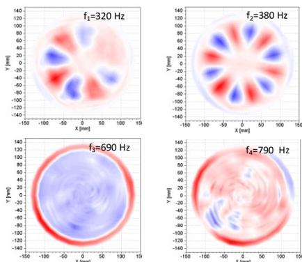
Figure 14: Vibration pattern of selected modes at natural frequencies  $f_1$ ,  $f_2$ ,  $f_3$  and  $f_4$  which generate significant 2<sup>nd</sup>-order harmonic input distortion ( $EHID$ ) in Figure 12.
