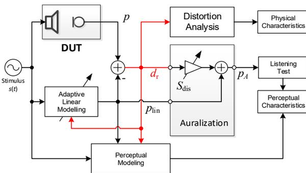
Figure 4: Evaluation of the loudspeaker while using typical guitar sound from the pickup as a stimulus.
