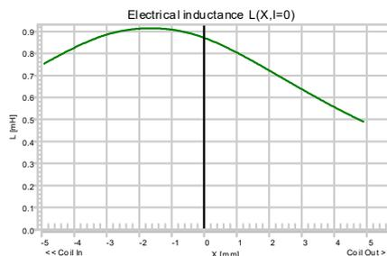
Figure 12: Voice coil inductance  $L(x)$  versus displacement  $x$ .
