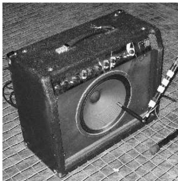
Figure 3: Loudspeaker cabinet in an anechoic chamber for near-field pressure response measurement.
